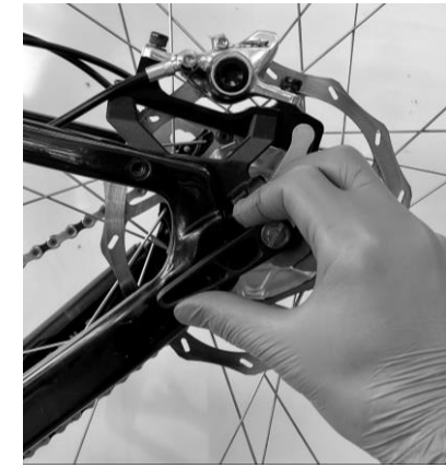
9.5: Tighten the thru-axle according to frame manufacturer specifications.
