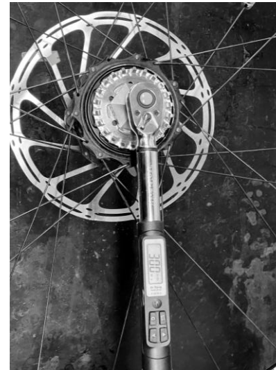
5.3: Torque the locking to 30 Nm.
