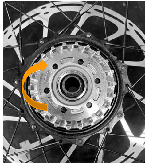
5.2: Install the hub sprocket locking by rotating clockwise.
