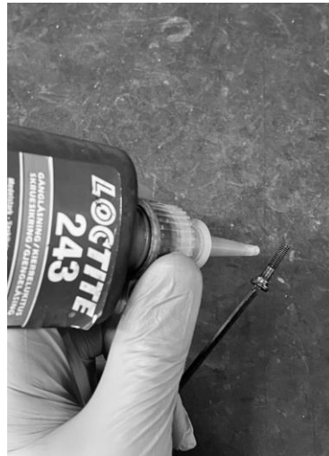
1.2: Apply Loctite 243 to the supplied SWAP bolts.
