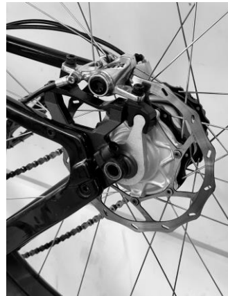
9.3: Align the torque arm and insert the wheel into frame.
