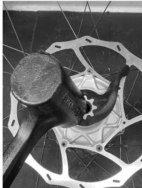
2.2: Gently tap the torque arm in place with a rubber mallet.
