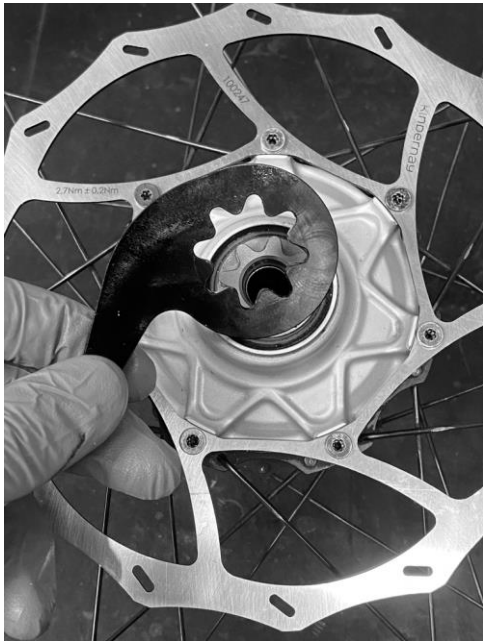
2.1: Align the torque arm with the flat face outwards, as shown.
