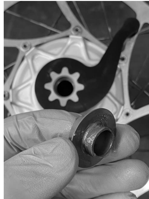
2.3: Lightly grease the end cap press fit surface.
