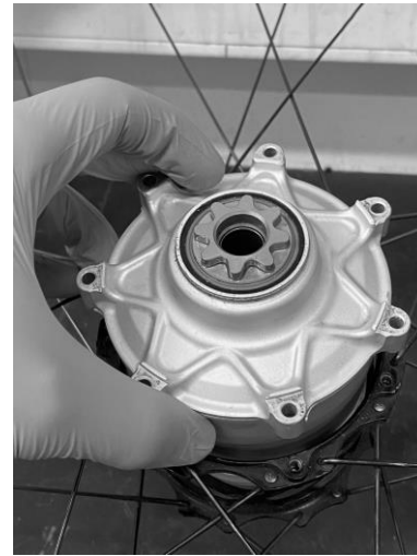
1.3: Install the gearhub in the SWAP.
