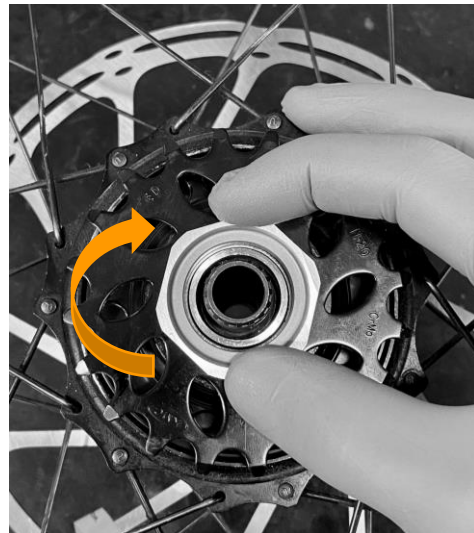
4.2: Install the hub sprocket locking by rotating clockwise.
