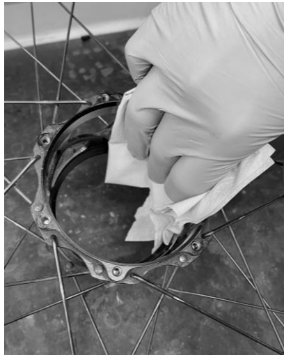
1.1: Clean the SWAP-shell and gearhub housing.
