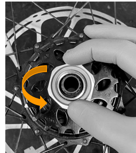
6.3: Remove the locking by rotating counterclockwise.
