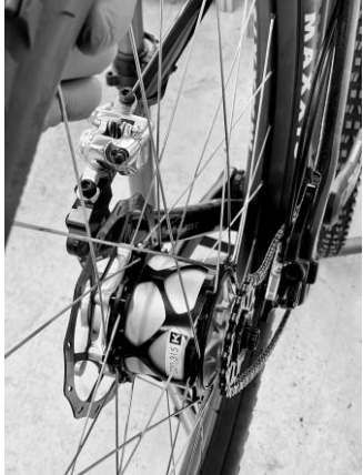
9.1: Install the chain/belt on the gearhub sprocket.
