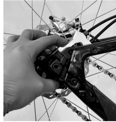
9.4: Install, but do not tighten the thru-axle. Position the actuator in the desired position.
