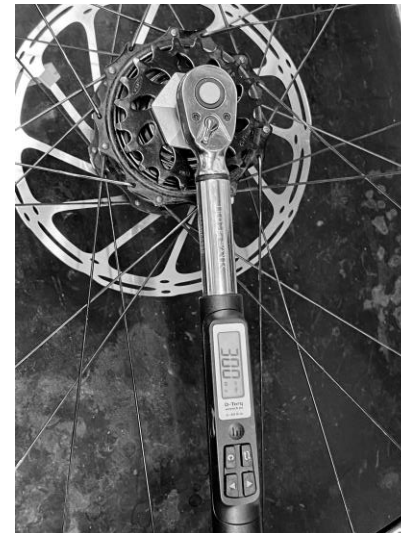
4.3: Torque the locking to 30 Nm.
