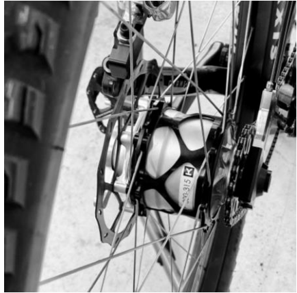
9.2: Install the actuator by pressing it on the drive side of the hub.
