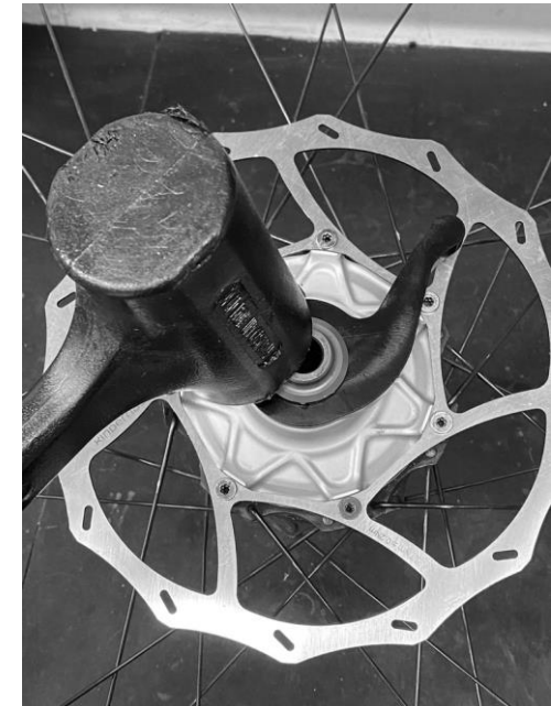
2.4: Gently tap the match cap in place with a rubber mallet.
