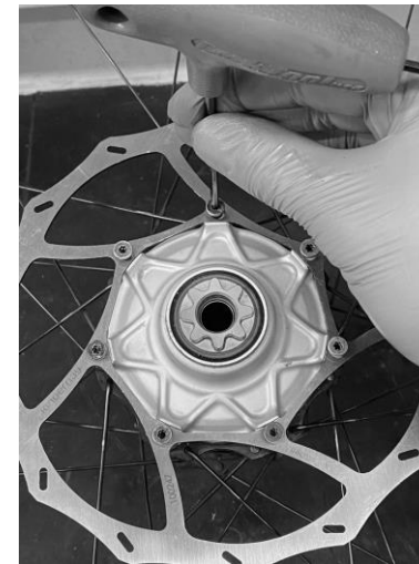
1.4: Install the brake rotor, align the bolt holes and install the bolts.
