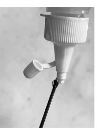
Thread locker: Using linseed oil will allow the nipples to rotate freely during tensioning, but seize up after a few days. This will reduce the likelihood of the nipples unwinding if the rim is damaged or bent.
