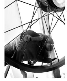
**De-stressing:** It is important to destress the spokes several times during tensioning. This will ensure the nipple and spoke are properly seated in the rim and SWAP cage, respectively.
