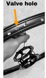
**1.2:** Pass the spoke through the spoke hole to the right of the valve hole.
