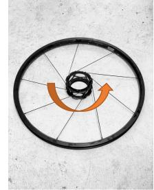
**1.5:** Complete the remaining spokes in a similar manner. Rotate the SWAP cage counter-clockwise, as seen from NDS to take up the initial slack.
