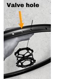
**1.2:** Pass the spoke through the spoke hole to the right of the valve hole.
