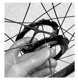
**4.1:** Install a spoke in any of the remaining DS flange holes, exiting on the outside of the flange.
