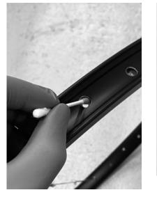
**Rimbed lubrication:** We recommend lubricating the rimbed slightly with Kindernay Velvet fluid, motor oil or other similar lubricant. This will allow the nipple to rotate more easily during tensioning.
