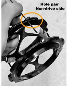
1.1: Insert a spoke in a nondrive side flange hole (the side with the threaded holes), through the left hole in the hole pair as seen from the drive side (as shown).
