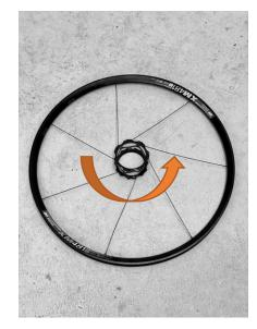
**1.5:** Complete the remaining spokes in a similar manner. Rotate the SWAP cage counter-clockwise, as seen from NDS to take up the initial slack.
