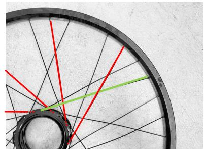
**4.2:** Route the spoke over the two first trailing spokes, and under the last trailing spoke. The spoke should be routed as shown, with trailing spokes in red and leading spoke in green.
