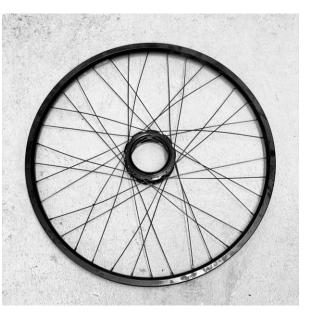
**4.3:** Repeat for the remaining spokes, completing the wheel lacing.
