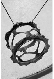
**1.3:** Pick the second next hole in the NDS flange and insert a spoke as in step 1.1.
