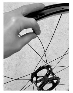
**3.2:** Carefully maneuver the DS spoke between the NDS spokes. It is ok to bend the spoke slightly in this process.
