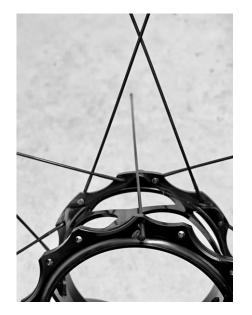
**3.1:** Insert a spoke in any drive side flange hole to the right of a NDS trailing spoke, exiting on the inside of the flange.
