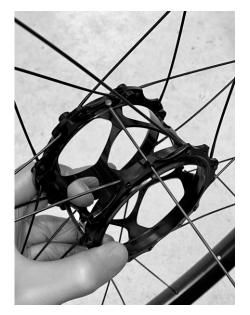
**4.1:** Install a spoke in any of the remaining DS flange holes, exiting on the outside of the flange.
