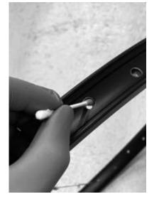
**Rimbed lubrication:** We recommend lubricating the rimbed slightly with Kindernay Velvet fluid, motor oil or other similar lubricant. This will allow the nipple to rotate more easily during tensioning.
