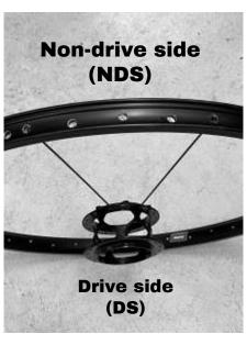
**1.3:** Attach the spoke from step 1.2 as shown, with 3 spoke holes in between.
