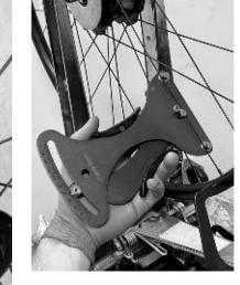
**Tensioning:** Ensure even spoke tensions to maximize the longevity of the wheel components.
