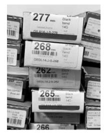
Spoke selection: We recommend using 1.8 triple butted spokes with 2.34 mm elbow diameter and brass nipples. Using thicker spokes will result in a less dynamic wheel, where spokes will loosen more easily.
