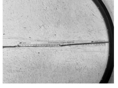
**1.1:** Cut two spokes to exactly 200 mm and attach them with a rubber band.
