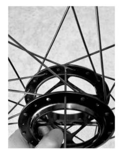
**4.1:** Install a spoke in any of the remaining DS flange holes, exiting on the outside of the flange.
