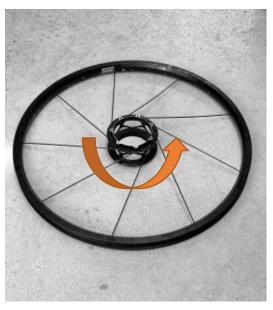
**1.4:** Complete the remaining spokes in a similar manner. Rotate the SWAP cage counter-clockwise, as seen from NDS to take up the initial slack.
