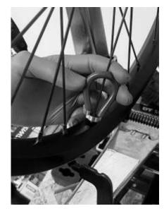
Tensioning: Be methodical in the tensioning process and pay attention to the spoke rotation to avoid spoke twist.
