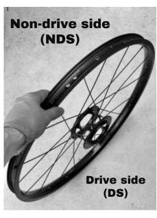
2.1: Install a spoke in any of the remaining NDS flange holes, exiting on the outside of the flange.
