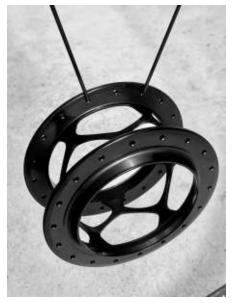
**1.2:** Pick the second next hole in the NDS flange and insert a spoke as in step 1.1.
