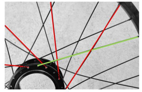
**4.2:** Route the spoke over the two first trailing spokes, and under the last trailing spoke. The spoke should be routed as shown, with trailing spokes in red and leading spoke in green.
