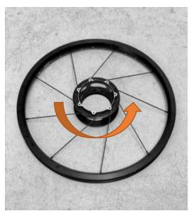
**1.4:** Complete the remaining spokes in a similar manner. Rotate the SWAP cage counter-clockwise, as seen from NDS to take up the initial slack.
