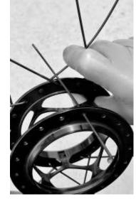
**3.1:** Insert a spoke in any drive side flange hole to the right of a NDS trailing spoke, exiting on the inside of the flange.
