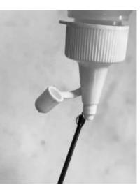
Thread locker: Using linseed oil will allow the nipples to rotate freely during tensioning, but seize up after a few days. This will reduce the likelyhood of the nipples unwinding if the rim is damaged or bent.
