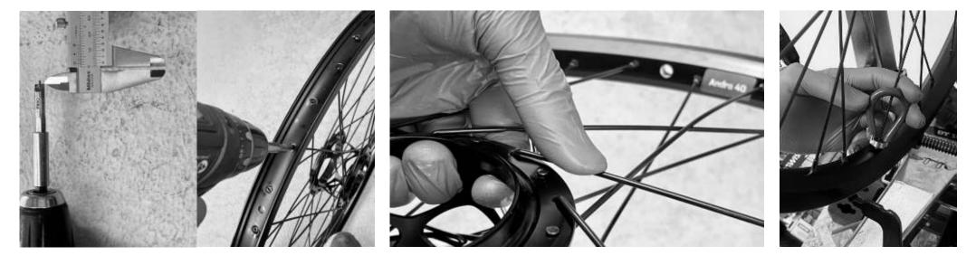
**5.1: (Optional)** Use a battery drill with a suitable spoke nipple bit to take up the initial slack. For most wheels, the limiter extension can be set to around 2 mm for the initial tensioning.
