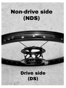
**1.3:** Attach the spoke from step 1.2 as shown, with 3 spoke holes in between.
