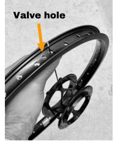
1.1: Insert a spoke in any of the non-drive side flange holes (the side with the threaded holes), exiting on the inside of the flange. Pass it through the spoke hole to the right of the valve hole.
