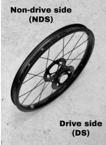
2.1: Install a spoke in any of the remaining NDS flange holes, exiting on the outside of the flange.
