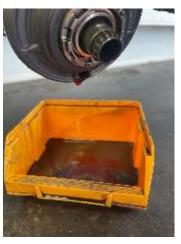
**1.2:** Position gear hub about suitable container with oil port down
