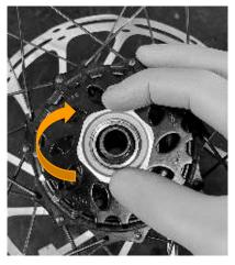
**4.2:** Install the hub sprocket lockring by rotating clockwise.
