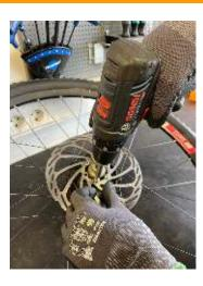
**1.3:** Remove brake rotor mounting bolts and rotor from hub
