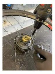
**1.4:** Remove gear hub mounting bolts
