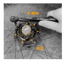
**1.4:** Tighten the bolts to 4 Nm in a star pattern. Repeat 3 times.
