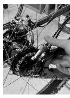
**9.4:** Install, but do not tighten the thru-axle. Position the actuator in the desired position.
