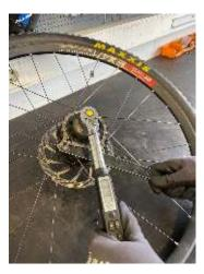
**1.2:** Remove drive cog from Hub using chain whip and 44mm GPC tool
