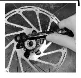
**2.3b:** Tighten the bolts to 6 Nm in a star pattern.
