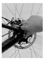
**9.5:** Tighten the thruaxle according to frame manufacturer specifications.
