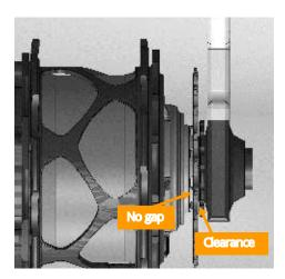
**4.4:** Verify that the HYSEQ actuator has clearance to the lockring and that there is not gap to the input shaft. The sprocket should rotate freely when the actuator is installed.
