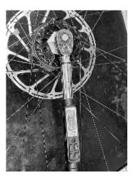
**4.3:** Torque the lockring to 30 Nm.
