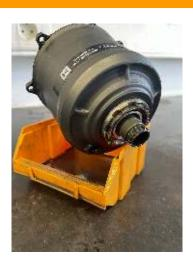
**1.3:** Allow gear hub to drain fully, appox. 5 minutes
